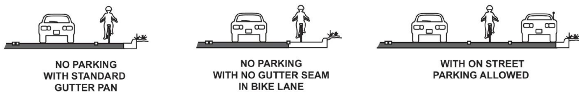
Figure A-5: Typical Roadways with Bike Lanes
