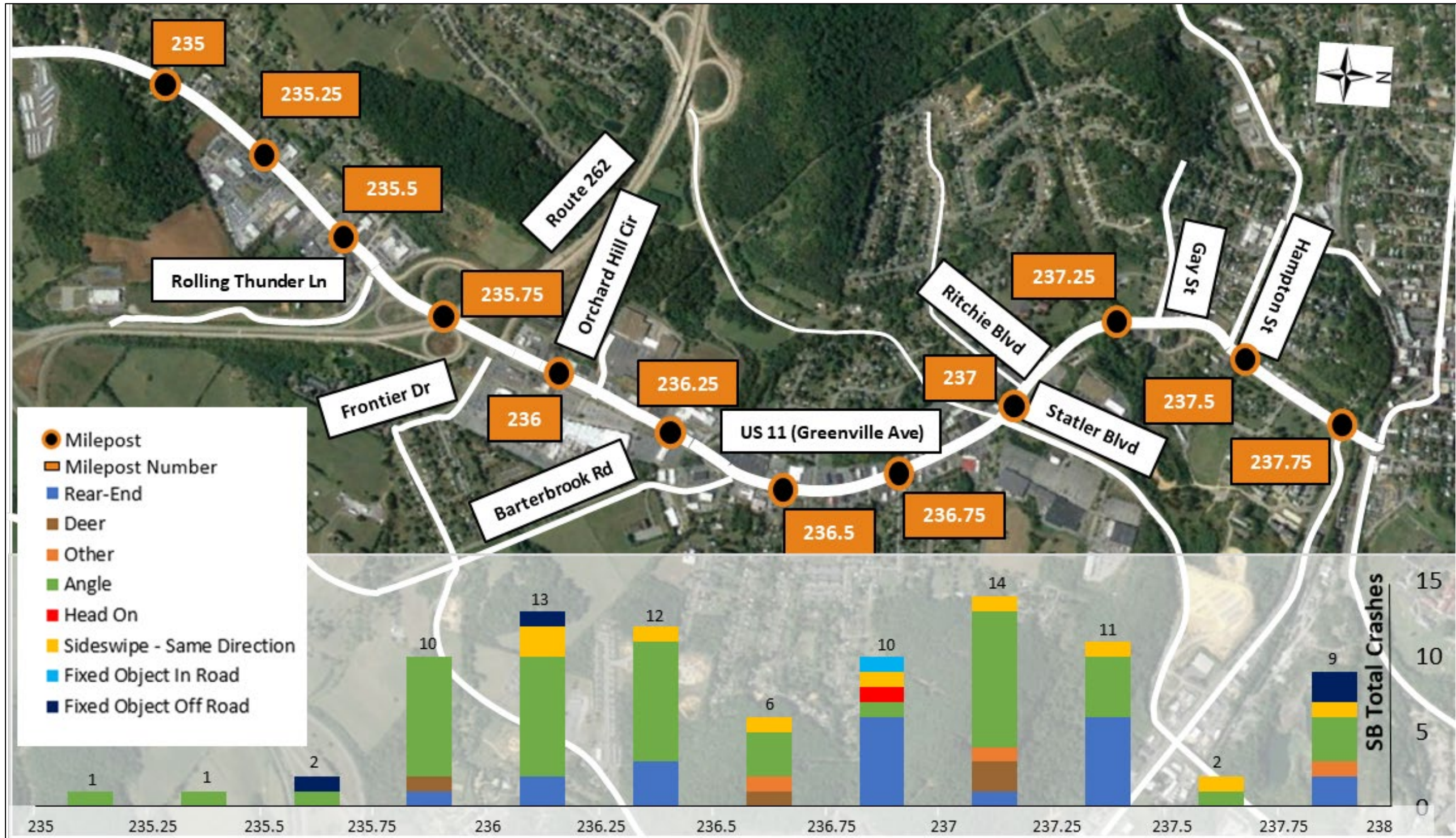
Figure 14: Crash Frequency by ¼ mile – Southbound US 11
