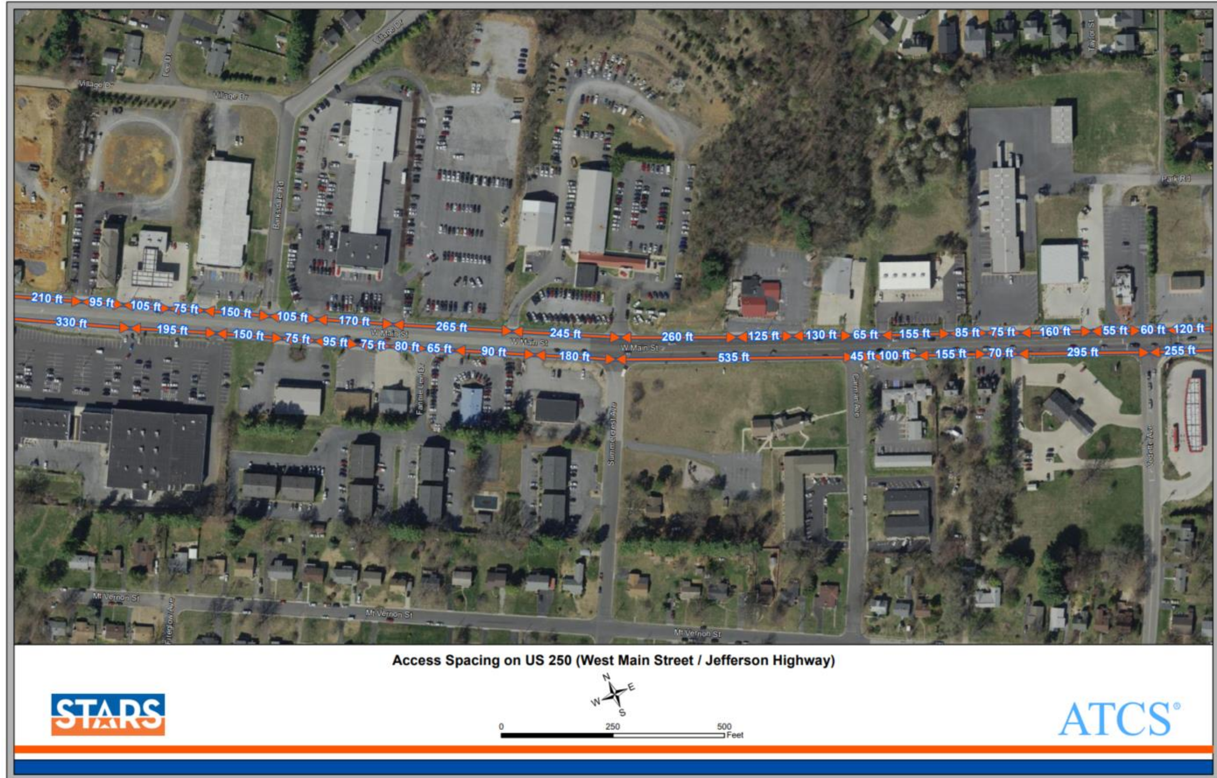
Figure 24: US 250 Existing Access Spacing
