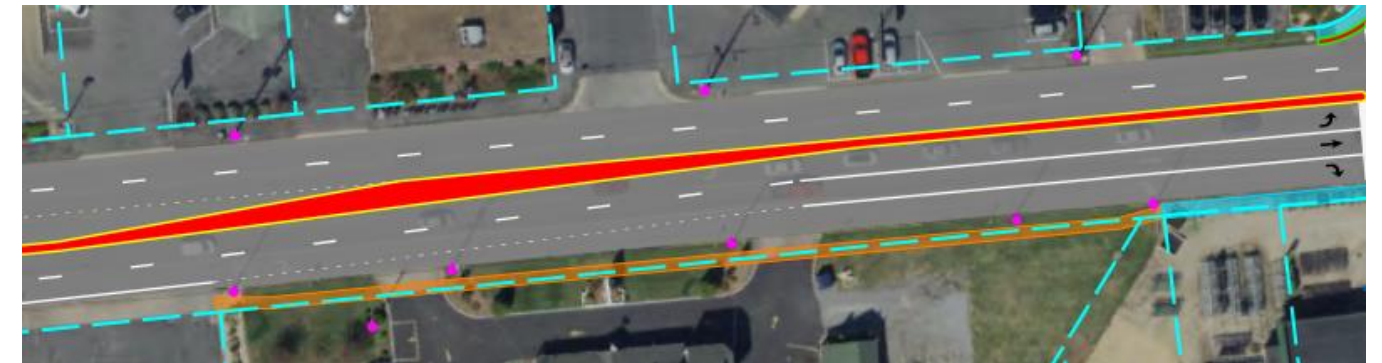
Figure 33: Proposed Lane Realignment on US 250 Eastbound Approach to Hopeman Parkway in Alternative 1
