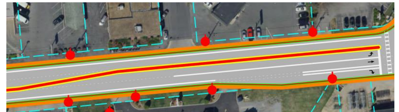
Figure 34: Proposed Lane Realignment on US 250 Eastbound Approach to Hopeman Parkway in Alternative 2
