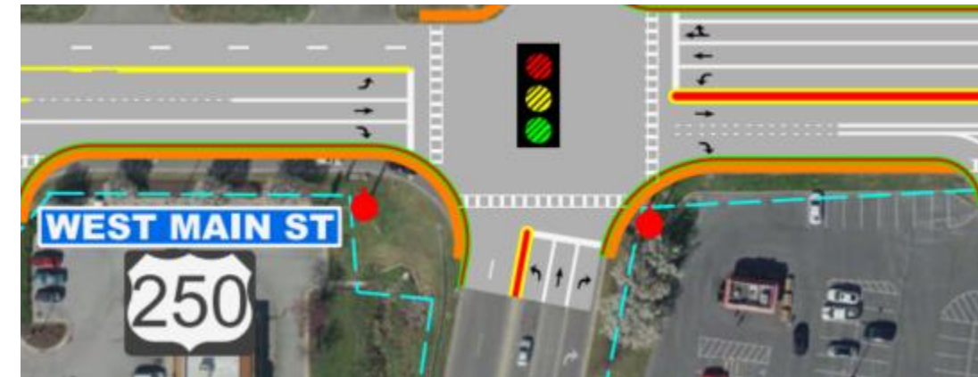
Figure 42: Revised Westbound Lane-Use at US 250 and Low Dewitt Boulevard/Pelham Drive for Alternative 2
