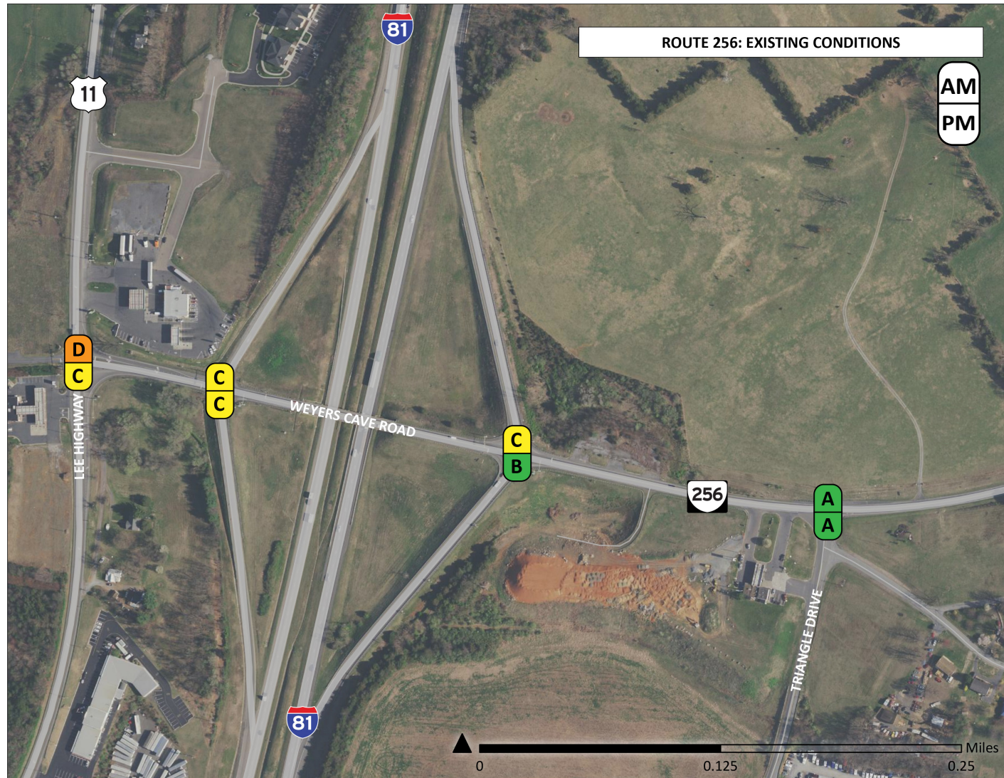
Figure 5. Intersection Level of Service Summary
