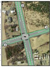
Route 250 at Route 636 Relocated and Wilson Complex 636-4-lane urban undivided 358-Extend right turn lane and add sidewalk/path 250 - Sidewalk/path additions with curb and gutter.
